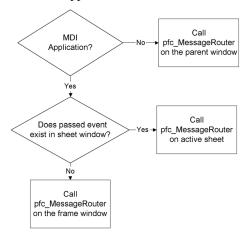
How pfc\_ MessageRouter works The pfc\_MessageRouter user event calls the passed user event in the window, the active control, and the last active DataWindow:
