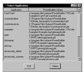
The Select Application dialog box displays a list of the applications defined in the Application section of the PB.INI file:
