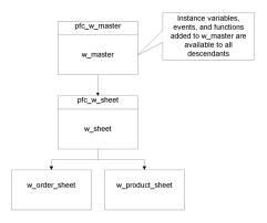
Adding extension levels The extension layer provides for reusability within an application and effectively insulates individual applications from PFC upgrades. But large installations that have department-wide (and perhaps corporate-wide) standards must extend this strategy further to implement additional levels containing corporate and departmental standards and business rules.
