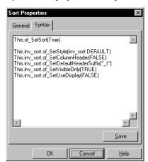
• Syntax Displays the PFC syntax used for the selected service:
