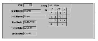
• Drop-down calculator for numeric or decimal values in an EditMask:
